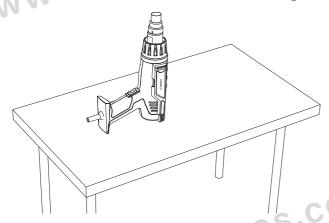
To let the heat tool cool down completely, push the switch to the position " — " and allow it to run for 2-3 minutes.
